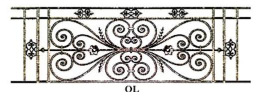
HT1 530mm HT2 460mm LG1 1600mm LG2 1370mm LG3 1200mm LG4 1100 mm
